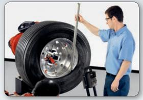
The standard hook tool is used to mount and demount tubed and super single tires or more difficult-to-handle wheel assemblies.
